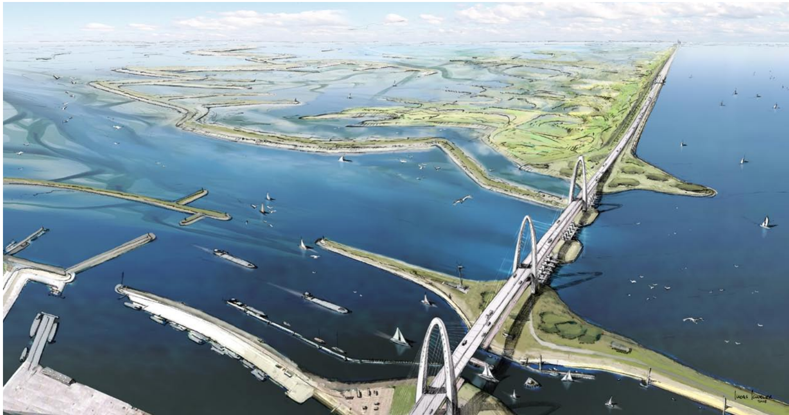
This new idea for the 36 km long Dutch seabarrier the 'Afsluitdijk' does not involve raising the height of the barrier, but establishes natural tidal marshes on the sea side, to bear the brunt of occasional storm surges.
