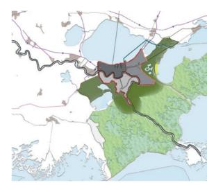
An example of the potential of Green Adaptation by Building with Nature for the Mississippi delta. Restoration of marshes could enhance the protection against storm surges and enhance the vitality of the local ecosystem. A comparable case in the Netherlands indicates that construction of a wave reducing marshland forest in front of a dike could be a safe, multifunctional and cost-effective solution.
