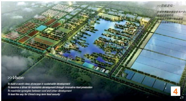
Figure 4: Artist's impression of Greenport Caofeidian in China, with residential areas, service areas and urban function areas in the middle surrounding a large water-storage lake. Greenhouses and closed fish production on the right, livestock production on the left and logistic functions top left and top middle.
